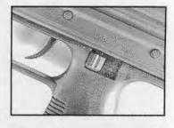
UZI-type selector bar on the left side of MP9's lower receiver blocks trigger when placed in the "SAFE" position. Movement of the selector forward from "SAFE" to "SEMI" and then to "AUTO" is in the ergonomically correct direction.
